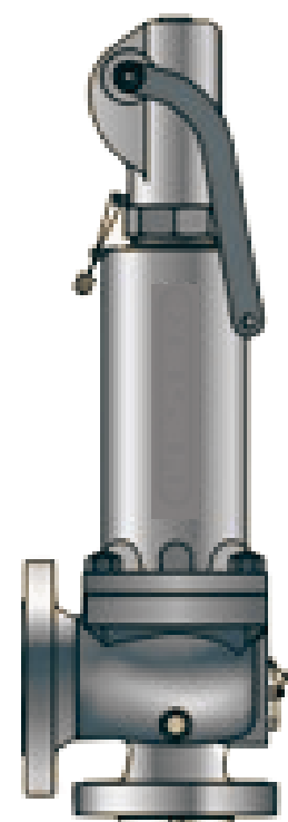
PACKED LEVER CLOSED BONNET CONVENTIONAL DESIGN
